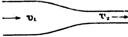
$$(h_1 + \frac{1}{2}v_1^2 + gz_1) - (h_2 + \frac{1}{2}v_2^2 + gz_2) - w + q = 0$$
