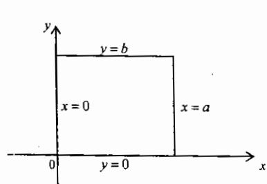
$$\frac{\partial^2 u}{\partial t^2} = c^2 \left( \frac{\partial^2 u}{\partial x^2} + \frac{\partial^2 u}{\partial y^2} \right) \quad (1)$$
